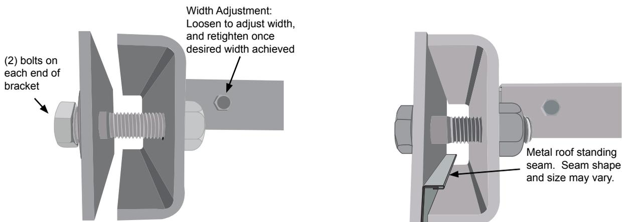
LOOSEN BOLTS ON EACH END OF DELUXE STANDING SEAM ROOF ANCHOR TO ALLOW FOR STANDING SEAM INSERTION INTO BRACKET.
